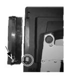
Take out the cable inside this cover as circled in the left picture here and connect it to connector inside the side mount upgrade kit as arrowed in the same
