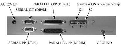
S1 Set security code. (Default Setting: BIT 1,2,3 OFF and BIT 4,5,6,7,8 ON. Security code is 07H)
