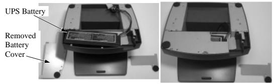
Place the optional UPS battery in the battery compartment in the way as indicated in the picture. Screw on the battery cover and join the battery cable into the cable routing operation. Please enable UPS function in software setting before use.
