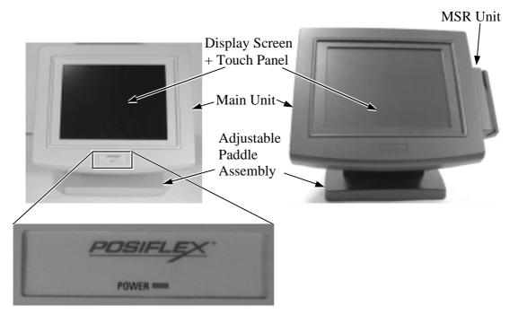
The MSR unit is option to both 12" and 15" models. The LED in the logo area serves for multiple purposes through giving different indication of steady/flashing green/orange light. Please refer to the paragraph discussing the LED indication in the chapter of "USING THE TOUCH POS" of this manual.
