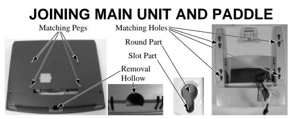
Match the matching pegs on the back of the main unit against one of the two sets of matching holes on the paddle. It is recommended to hook on the lower set of holes for better stability. First aim the matching pegs toward the upper round part of
