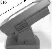
In order to settle the touch terminal properly in a point of sale system, all the cable connections have to be routed through its base, the paddle assembly. Therefore, please press the lock/release button at the rear side to separate the main unit from the paddle assembly.
