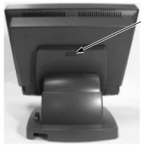
Press the Lock/Release button and lift the main unit to detach it from the paddle assembly.
