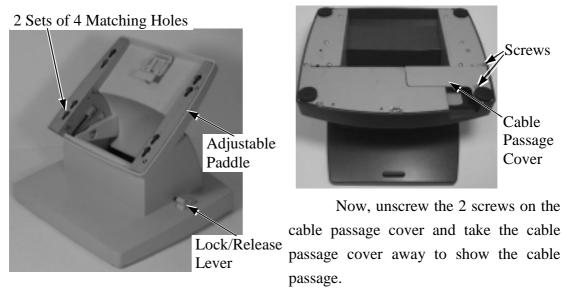
If there is no need to install the optional UPS battery here (either not to be installed or already installed), please skip the next paragraph and directly start routing cables through the cable passage. Otherwise, please remove the four screws holding battery cover to install the battery.
