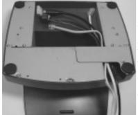
Place all the cables required for connections to the TP6000 series except those for special application purposes into the cable passage. Inset one end of the cable passage cover under the battery cover and screw on the two screws. Be sure not to damage any of the cables during this operation.
