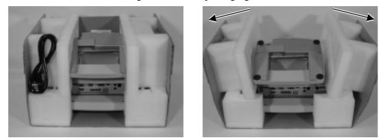
Take out the accessories/options from the partitions in the packaging materials and unfold the packaging materials carefully to unload the upsidedown loaded TP6000 series touch terminal. Put this main unit & paddle assembly aside for the whole Touch POS system installation. Collect if exist other options from the hidden compartments in the packaging materials like external FDD.
