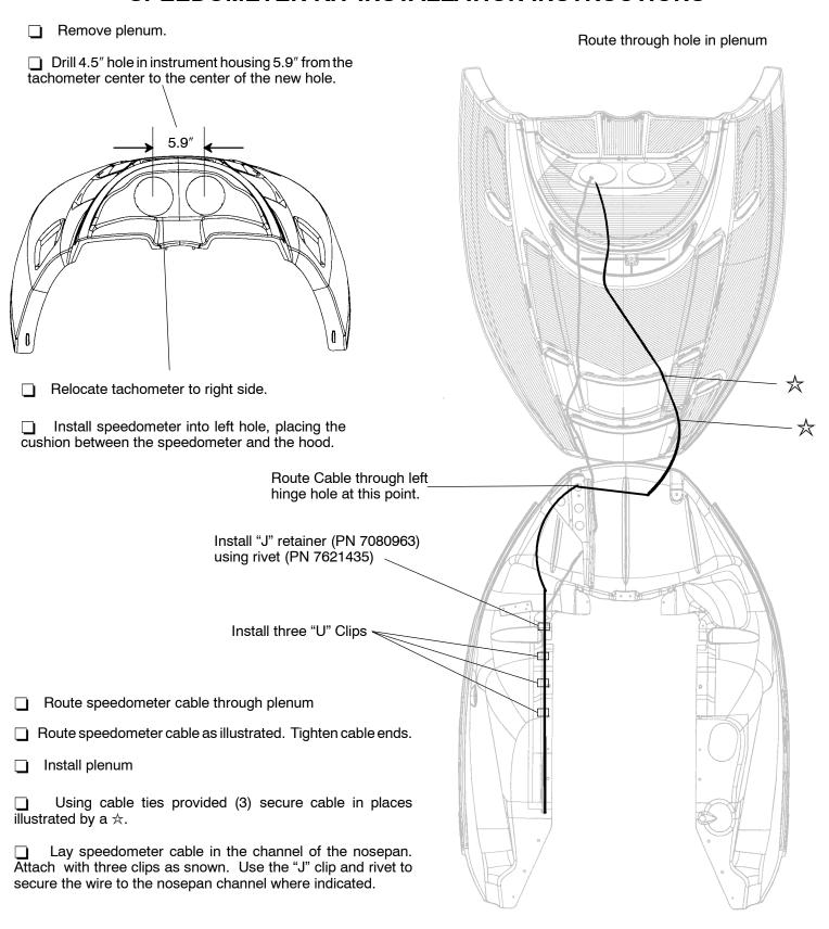
Dark line indicates speedometer cable routing.
