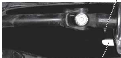
Fitting Access (as viewed from top with center floor panel removed)
