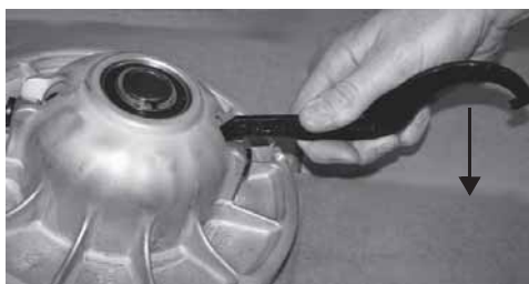
Apply force to opposite end of tool to spread sheaves.
