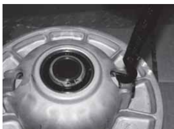
Insert hooked end of tool.
