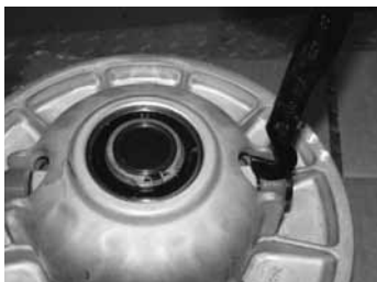
Insert hooked end of tool.
