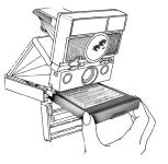
3 Close the film door. The camera will automatically eject the film cover and the electronic flash will begin to charge.
