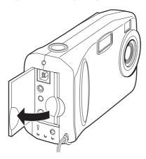
3 Insert the memory card into the slot (with the label side of the card facing the rear of the camera).
