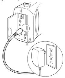
**2** Connect the other end of the cable to a grounded electrical outlet.
