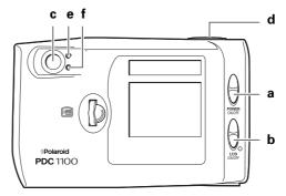
**4** Press the shutter button (**d**) halfway to focus the camera and measure the light level. The camera is ready to take a photo when the green LED indicator lights (**e**). Press the shutter button all the way down to take the photo.
