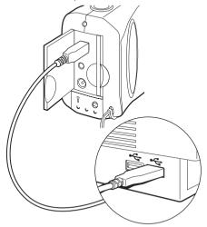
**2** Connect the rectangular USB cable to the USB port on the computer.
