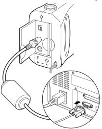
**3** Connect the serial cable to the serial port on the back of your computer.
