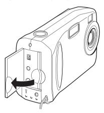
**3** Carefully insert the memory card into the slot. The card fits only one way.
