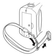
The wrist strap includes a clip to use when removing the memory card from the camera.
