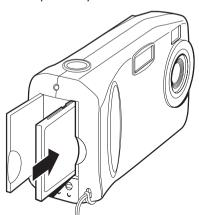
Make sure the card is pushed firmly into the slot.
