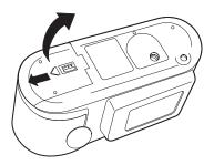
**2** Insert four AA-size batteries.
