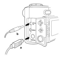
**Note:** Insert the connector straight into the digital port without twisting, so that the flat side of the connector (the side with the arrow on it) faces toward the back of the camera. If you encounter resistance, do not force the connector, but reposition it and try again.
