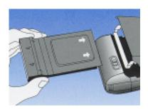
Close the film door; the film cover will advance automatically into the storage compartment and the counter will advance to 10. (The picture counter counts down, indicating the number of pictures left.)
