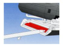
the film pack first. Insert the tip of a ballpoint pen into the small square in the red bar as shown. Pivot the red bar out of the way for access to both rollers. Clean the rollers with a lint-free cloth or a cotton swab dampened with water while manually turning the roller gear with your finger.
