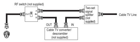
"A" position on the RF switch (not supplied): You can view all unscrambled channels by using the TV's channel keys.
