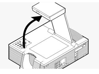
6 Locate the flip-mirror-release lever on the top of the arm. Slide it in the direction of the arrow while pulling up on the lift tab. This releases the mirror.
