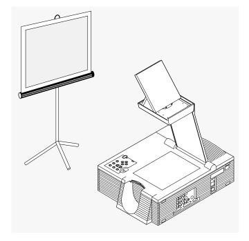
*3* The projector must be parallel to the floor. If you use a media cart, make sure the wheels are locked to prevent it from moving.
