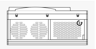
6 Locate the thumbscrew on the right side of the lamp and unscrew it. When the thumbscrew is loose enough, gently pull the lamp from the right socket. Then slide it out from the left.
