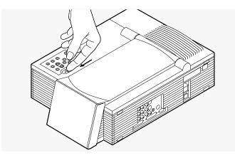
*Sliding the lever to release the arm*
