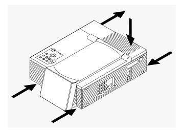
*Caution:* The lamp chamber gets very hot during operation, especially the ceramic sockets at each end of the lamp. Be careful when you open the lamp chamber or change the lamp. To allow that area to cool down, press the <sup>①</sup> button to turn off the lamp and let the fan cool the projector for at least five minutes before you touch any of those components. See Chapter 5, *Maintenance*, for more information. *Turning the lamp on and off*
