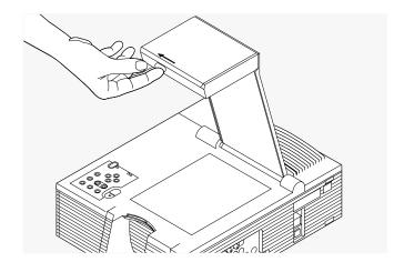
The flip-mirrorrelease lever 7 Gently tilt the flip mirror open approximately 45° (you can adjust the angle of the mirror later, to raise or lower the projected image).
