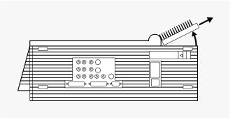
The filter is located on the inside of the top left cover (see the illustration below).
