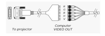
*3* Connect the optional Polaview BNC-to-LCD connector cable (part number C803-6) to the projector COMPUTER OUT connector and the monitor BNC video input. Use the same BNC connections used with the monitor.
