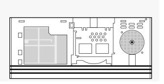
Remove the retaining screw to gain access to the filters. Pull the front filter out
