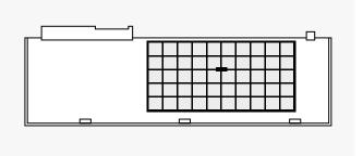
4 There is a plastic grill covering the filter. Pull on the handle in the center of the grill to access the filter.
