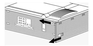
5 Locate the door to the lamp chamber on the right side of the left panel. It has one slotted, captive screw. With a screw-driver or coin, loosen the screw, then open the lamp-chamber door.
