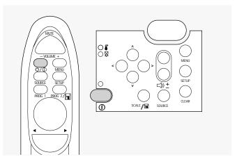
To turn the lamp off, press and hold the ① key for about two seconds. When you turn the lamp off, the projector fans continue to run for about two minutes. Allow the fans to run until they automatically turn off. This lengthens the lamp life and helps ensure that the projector cools properly. Turning the lamp off does not turn off the projector. To turn the power off, move the power switch on the back of the projector to the "off" position.
