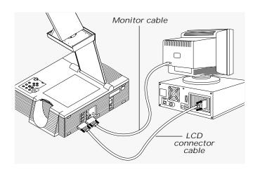
Silicon Graphics 13C3 video connections If you have a Silicon Graphics workstation with 13C3 connectors at the computer and monitor video ports:
