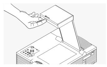
6 Gently tilt the flip mirror approximately 45°. (You can adjust the angle later to raise or lower the projected image.)
