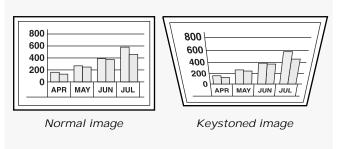
Keystoning occurs when the front of the projector is not perpendicular to the projection screen (the vertical plane) or when the projector is not parallel to the floor (the horizontal plane). Keystoning can also occur when the projector is tilted sideways.
