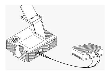
The composite audio/video cable (part number C497-6) has a yellow, red, and white RCA plug at each end. To connect an NTSC, PAL, or SECAM source to your projector, make the appropriate cable connections, as indicated in the following chart:
