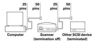
You may need additional cables or adapters to connect the scanner. Your cable must have a 50-pin Centronics M or DB-25 M connector at one end for attachment to the scanner, and the cable should be as short as possible. To determine the connector you need for attachment to your SCSI adapter, refer to instructions with the adapter.
