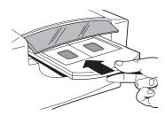
**3** Close the carrier access door. The scanner will not scan if the door is open.
