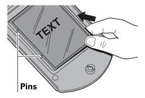
**3** Close the carrier. Squeeze the carrier at the bottom edge and turn the knob to lock it.
