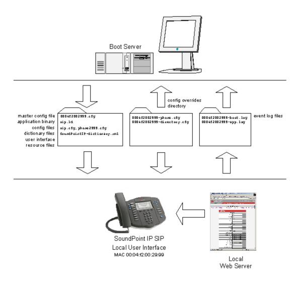
A boot server allows global and per-phone configuration to be managed centrally through XML-format configuration files that are downloaded by the phones at boot time. The boot server also facilitates automated application upgrades, diagnostics, and a measure of fault tolerance. Multiple redundant boot servers can be configured to improve reliability.
