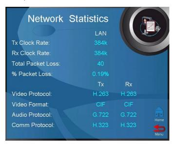
**Tx Clock Rate** Transfer clock rate; the clock rate for outgoing
