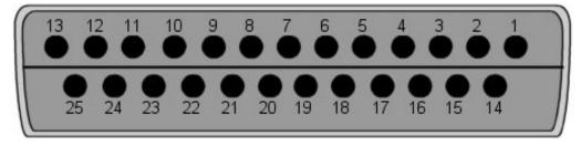
The Logic Output port is a female DB-25 connector where pins 1-20 can be programmed. Pins 21-25 are ground pins. Each pin can source up to 20 mA of current and each ground pin can sink up to 100 mA of current.
