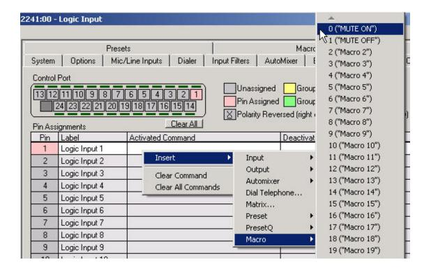
Now, right click in the DEACTIVATED COMMAND column for Logic Input 1 and select INSERT, MACRO, 1 "(MUTE OFF"). Now, whenever the switch goes Active High (+ 5V DC), the Vortex Device will execute Macro 1.
