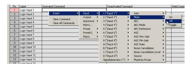
Now, right click in the DEACTIVATED COMMAND column for Logic Input 1 and select INSERT, INPUT, 1, MUTE, ON. Now, whenever the switch goes Active High (+ 5V DC), the Vortex Device will mute Input 1.
