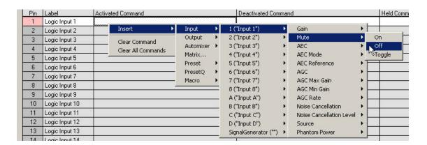
Now, right click in the DEACTIVATED COMMAND column for Logic Input 1 and select INSERT, INPUT, 1, MUTE, ON. Now, whenever the switch goes Active High (+ 5V DC), the Vortex Device will mute Input 1.
