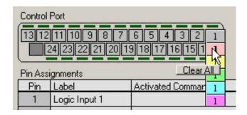
Now, right click in the ACTIVATED COMMAND column for Logic Input 1 and select INSERT, INPUT, 1, MUTE, ON. Now, whenever the switch goes Active Low (OV DC), the Vortex Device will mute Input 1.
