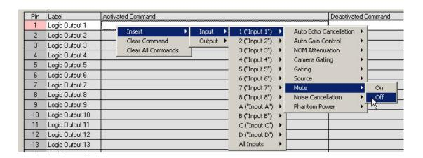
Next, right click in the DEACTIVATED COMMAND column for Logic Input 1 and select INSERT, INPUT, 1, MUTE, ON. Now, whenever the microphone is muted (Mute = True), the LED will not illuminate on the MX392.
