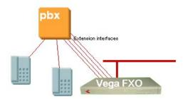
When making calls from VoIP to PBX the dialled number is passed using DTMF tones played into the PBX.
