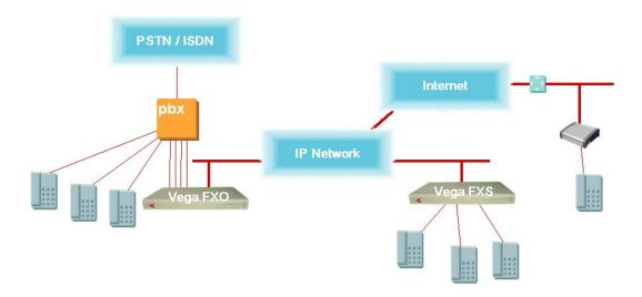
When expanding into new offices it can be expensive and inconvenient to set up a new PBX or run analog leased lines from the main site to the new remote site. Data infrastructure between sites however is essential. Keeping the Main site PBX for all users brings many benefits, including extension number dialling to all personnel, voice mail on a single site, common functionality for all phone users (people can move offices and do not have to learn a new phone system).
