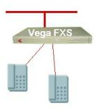
Analog telephones can be connected directly into the Vega FXS ports. This allows existing or new (and often cheap) analog telephones to be connected into a VoIP system. This can be especially useful where Cat 5 cabling already runs analog phones to peoples' desks; the Vega can replace the PBX in the telecoms cabinet, the Cat 5 telephone extensions terminate on the Vega FXS rather than on the old PBX.
