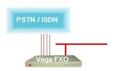
A Vega FXO can be connected directly to PSTN lines.
