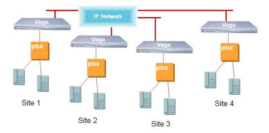
In larger companies, the PBXs on multiple sites may be linked together via leased lines and using QSIG signalling in order to make the distributed PBXs function as though they were a single PBX.
