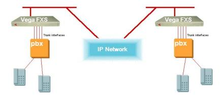
Out-dialled calls from the PBX can pass a dialled number to the Vega; it can use this to decide which destination VoIP gateway to route the call to (i.e. multiple destination gateways may be supported).
