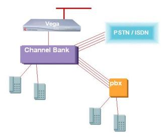
Where mass capacity of FXS and / or FXO interfaces are required it can be cheaper to use a Vega 400 together with a channel bank.
