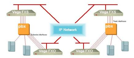
In this configuration calls may be routed PBX to FXS to FXO to PBX or PBX to FXO to FXS to PBX.
