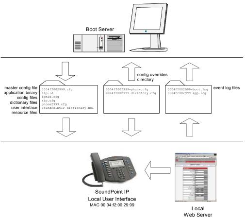
A boot server allows global and per-phone configuration to be managed centrally via text XML-format configuration files that are downloaded by the phones at boot time. The boot server also facilitates automated application upgrades, diagnostics, and a measure of fault tolerance.
