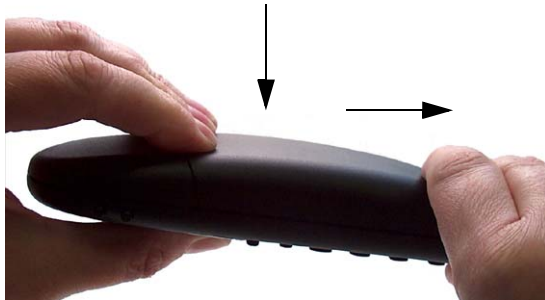
Figure 1 Remove Back Cover from Handset
