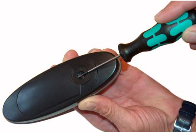
Figure 10 Remove Back Cover from Handset with Screw Fastener
