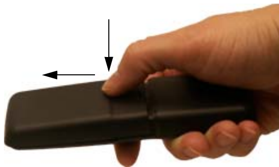
Figure 11 Remove Back Cover from Handset
