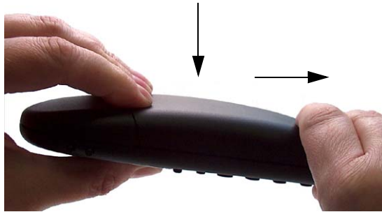
Figure 9 Remove Back Cover from Handset
