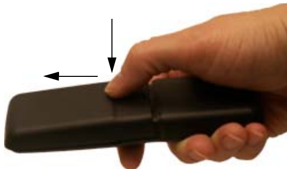
Figure 3 Remove Back Cover from Handset
