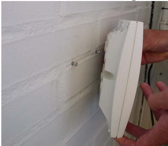
Figure 11 Wireless Server 600v3 Wall Mounting
