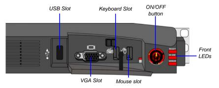
Figure 1-2 RMX 1500 Front Panel
