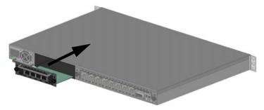
4 Insert the card into the slot and tighten the captive screws on each side of the rear panel of the card, securing the RTM ISDN card to RMX.
