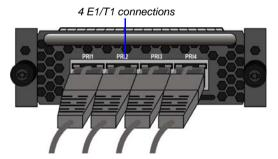
Figure 1-4 RMX 1500 RTM ISDN Rear Panel Layout
