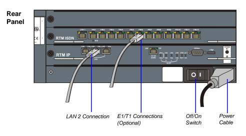
Do not remove the protective plastic caps from LAN1, LAN3 and ShMG ports.
