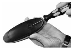
To remove the batter cover, use a normal screw driver. Insert it into the small crack behind the blind cover and break to open the handset.
