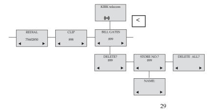
Storing a number (ma . 24 digits) in the telephone book is done b pressing the number to be stored (in on hook), then press the > -ke followed b the \( \strick \)-ke . The book can store up to 200 numbers with name. T ping of the name and a confirmation is required. After storing the telephone will go back to standb mode. If the displa shows
