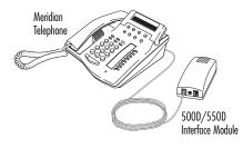
Any digital phone supported by your telephone network can be connected to the phone jack on the 500D/550D Interface Module.
