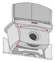
2. Focus the camera using the focus wheel:
