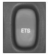
To turn the system on or off, press the ETS button on the located on the left side of the instrument panel near the instrument panel brightness control.
