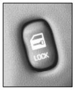
You can lock or unlock all doors of your vehicle from the driver's or front passenger's door lock switch.
