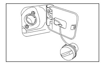
While refueling, hand the cap inside the fuel door by placing the fuel cap strap in the strap hanger.
