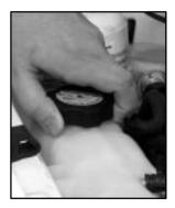
5. Then replace the pressure cap. Be sure the pressure cap is hand-tight.
