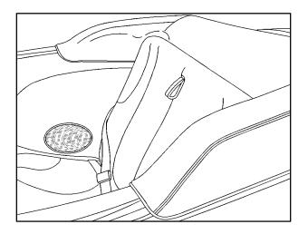
5. Raise the rear seatback to the up position. Push the seat back to make sure it is latched.
