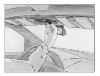
6. Rotate the latch handle up to the locked position.
