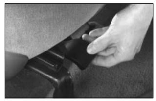
If your vehicle is equipped with easy entry seats, this is your front passenger seat adjuster. Pull up on the lever at the front of the seat to unlock it. Slide the seat to a comfortable position. Release the lever and try to move the seat with your body, to make sure the seat is locked into place.
