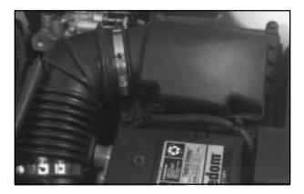
The air cleaner is located on the driver's side of the engine compartment near the battery.
