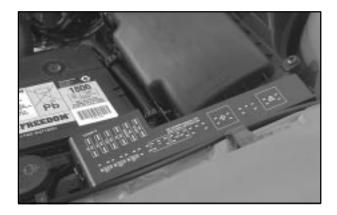
The engine compartment fuse block is located on the driver's side of the engine compartment. Lift the cover to check the fuses.
