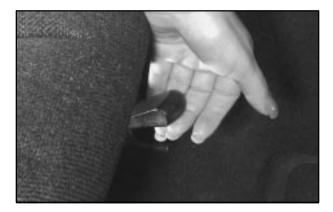
If your vehicle is not equipped with easy entry seats, your passenger seat adjuster looks like this. Slide the lever under the passenger's seat to the right to unlock it. Slide the seat to where you want it. Then release the lever and try to move the seat with your body, to make sure the seat is locked into place.
