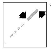
3. Check both sides of the dipstick, and read the lower level. The fluid level must be in the cross-hatched area.
