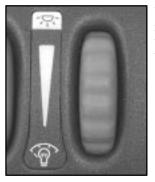
You can brighten or dim the instrument panel lights by turning the thumbwheel up or down.
