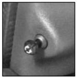
The mirror control is located on the driver's door. Turn the control clockwise or counterclockwise to choose the mirror you want to adjust.
