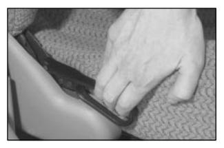
To adjust the seatback, lift the lever on the outer side of the seat and move the seatback to where you want it. Release the lever and push rearward on the seatback to make sure it is locked. Pull up on the lever and the seat will go to an upright position.
