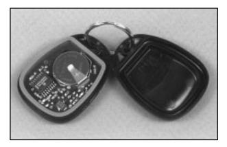
To replace the battery in the transmitter:
