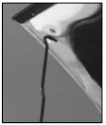
Lift the hood, release the hood prop from its retainer and put the hood prop into the slot in the hood marked "PROP ROD."
