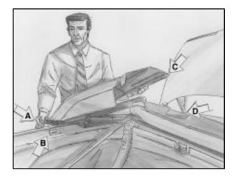
3. Install the boot side cover by inserting the tab (A) on the underside of the cover into the slot (B) at the top of the quarter trim panel. Place the rear flap of the boot side cover in the trunk lid opening, aligning the eyelet (C) over the boot snap ball stud (D). Repeat this step for the opposite side boot cover.
