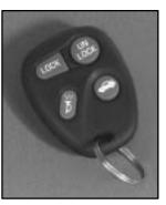
The remote keyless entry system consists of a receiver, which is located in the vehicle, and two hand held transmitters. Your remote keyless entry system operates on a radio frequency subject to Federal Communications Commission (FCC) Rules and with Industry Canada.
