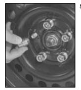
8. Reinstall the wheel nuts with the rounded end of the nuts toward the wheel. Tighten each nut by hand until the wheel is held against the hub.
