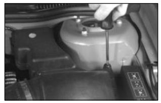
To check or replace the filter, remove the screws that hold the cover on and lift the cover. Be sure to reinstall the air cleaner filter and reinstall the cover tightly.
