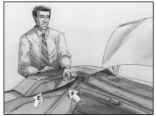
4. Attach the two snaps on the inside flap of the side cover, to the side of the quarter trim panel. Attach the front snap (E) first and then the rear snap (F). The rear snap is adjustable for ease of installation. Repeat this step for the opposite side boot cover.
