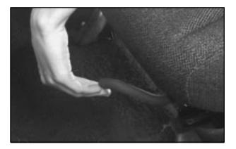
Lift the lever under the driver's seat to unlock it. Slide the seat to where you want it. Then release the lever and try to move the seat with your body, to make sure the seat is locked into place.
