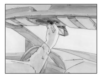
6. Turn the latch handle up to lock the top. Be sure the top is securely latched on both sides.
