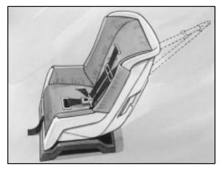
In Canada, the law requires that forward-facing child restraints have a top strap, and that the strap be anchored. In the United States, some child restraints also have a top strap. If your child restraint has a top strap, it should be anchored. If you have a convertible, don't use a restraint like that in your vehicle because the top strap anchor cannot be installed properly. You shouldn't use this type of restraint without anchoring the top strap.
