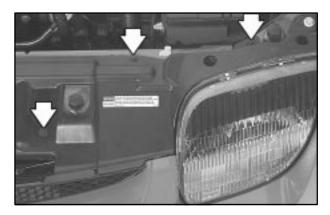
1. Remove the six plastic fasteners holding the shield. Use the end of a flat-head screwdriver to pull up the center of the fastener. Be careful not to break the fasteners that hold the shield in place.
