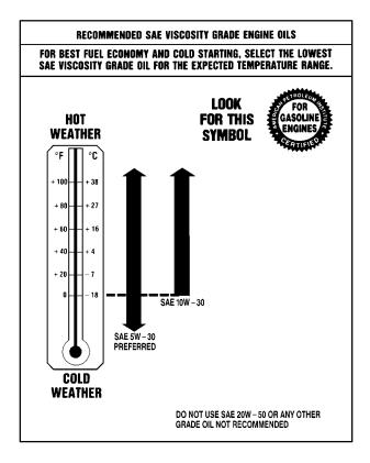
As shown in the chart, SAE 5W-30 is best for your vehicle. However, you can use SAE 10W-30 if it's going to be  $0^{\circ}$ F (-18°C) or above. These numbers on an oil container show its viscosity, or thickness. Do not use other viscosity oils, such as SAE 20W-50.
