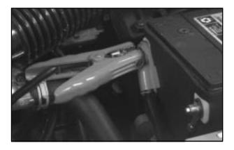
Remove the red plastic cap, and connect the red positive (+) cable to the positive (+) terminal of the vehicle with the dead battery. Use a remote positive (+) terminal if the vehicle has one.
