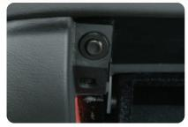
For added security, the trunk release button is disabled when all the doors are locked using the Remote Keyless Entry transmitter LOCK button or through the door lock knob.
