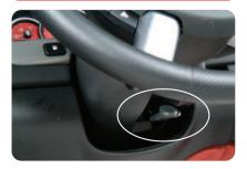
To adjust the steering wheel position, locate the adjustment lever under the steering column. Hold the steering wheel and rotate the lever down; then move the steering wheel to the desired position (the wheel can be adjusted up/down and in/out). Rotate the lever back up to lock the steering wheel in place.
