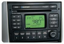
Setting the Time: With the radio on, press the TIME button for more than two seconds. When TIME ADJ or SET TIME is displayed, press the SEEK/TRACK arrows to adjust the hours. Press the TUNE arrows to adjust the minutes, and then press the TIME button again to save the setting.
