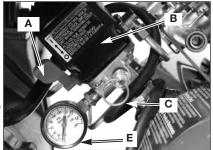
**Safety Valve (C):** If the pressure switch does not shut off the air compressor at its "cut-out" pressure setting, the safety valve will protect against high pressure by "popping out" at its factory set pressure (slightly higher than the pressure switch "cut-out" setting).
