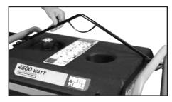
With skyhook resting on fuel tank install upper bracket as shown.
