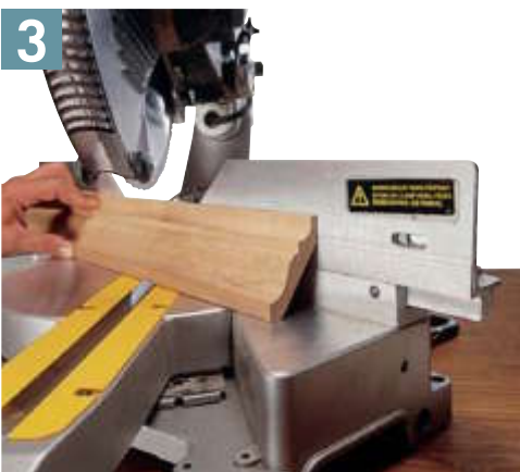
A tall fence makes it easier to cut crown molding.
