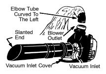
When converting back to the blower feature, make sure that the latch on the vacuum inlet cover is securely fastened.
