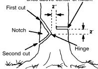
After removing the wood from the notch, make the felling cut on the opposite side of the notch. This is done by making a cut about two inches higher than the center of the notch. This will leave enough uncut wood between the felling cut and the notch to form a hinge. This hinge will help prevent the tree from falling in the wrong direction.
