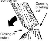
**NOTE:** Before felling cut is complete, use wedges to open the cut if necessary to control the direction of fall. To avoid kickback and chain damage, use wood or plastic wedges, but never steel or iron wedges.
