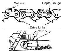
Place chain onto the sprocket
