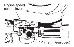
MODELS WITH FIXED SPEED ENGINES Engine speed was set at the factory for optimum performance. Engine speed is not adjustable.
