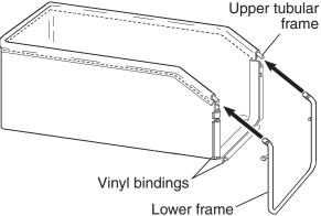
ASSEMBLE TOP TO FRAME AND BAG **NOTE:** For ease of assembly, place catcher top upside down on work surface.
