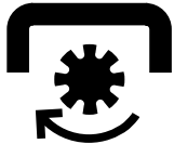
ATTACHMENT CLUTCH ENGAGED
