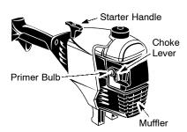
WARNING: The trimmer head will turn while starting the engine. Avoid any contact with the muffler. A hot muffler can cause serious burns.
