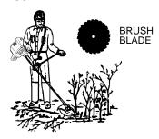
**NOTE:** If your unit has been assembled for trimmer head use, refer to the section ATTACH-ING THE PLASTIC SHIELD AND TRIMMER HEAD and reverse the steps to remove the plastic shield and trimmer head before you mount the metal shield and blade. Store these parts for future use. Never use the trimmer head with the metal blade installed.
