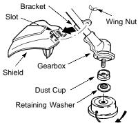
**NOTE:** Make sure all parts are properly installed as illustrated in the illustration before installing the trimmer head.
