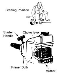
**WARNING:** The trimmer head will turn while starting the engine. Avoid any con-tact with the muffler. A hot muffler can cause serious burns.
