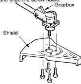
Insert the 4 mounting screws through the bottom of the shield. Thread them into the gearbox. Tighten evenly and securely with one of the hex key wrenches provided.
