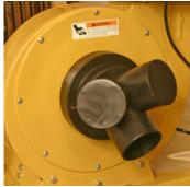
The smooth surfaces and curves of the sheet metal chute (left) enhance airflow and efficiency. This triple 4"-outlet adapter (right) slips onto an 8"-diameter port to provide the most versatility in your shop.
