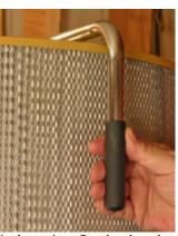
A pair of "hands" (left) within the canister flex the pleated element to knock off excess buildup. The hands are operated by the external handle (right), which is generally turned through one revolution per month in most home woodshop circumstances.
