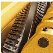
The sophisticated helical head creates ultra-smooth surface with far less cutter replacement or maintenance than with conventional knife systems.
