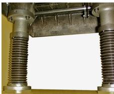
The table has gib adjustments (left) at either side to eliminate play that might develop over the years. Each of the massive lead screws has an adjusting collar at its top (right) to keep the table parallel to the cutterhead.
