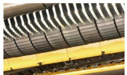
The segmented feed rollers make working with various thickness pieces safe and consistent. The result is higher production without sacrificing quality.
