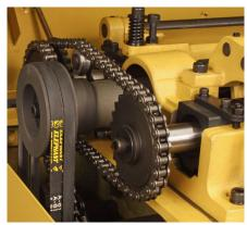
The twin in-bed rollers are adjustable from the front of the PM201HH (left) so these changes can be made quickly without disturbing cut depth. The cutterhead is powered by a dual belt and the rollers with a slip-free chain drive. (right)
