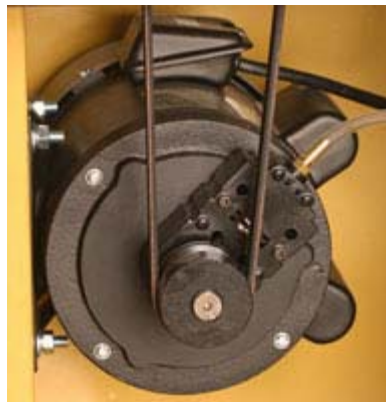
The motor (left) is pre-installed in the enclosed base and sends its power through machined pulleys and an ultra-reliable Poly V-belt. The 9-spoke cast iron drive wheels (right) are fully machined, painted and fitted with tires before being dynamically balanced.
