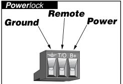
the vehicle, it is time to connect the wires to the **DAC-348**. Be sure that you have not reconnected the ground cable to the negative post of the battery.
