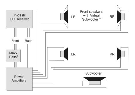
**WARNING:** If you are using a source unit with bridged high powered (or "floating ground") speaker outputs, a suitable high to low level adapter must be used. If you are unsure about your head unit see your local *PrecisionPower*<sup>TM</sup> dealer.
