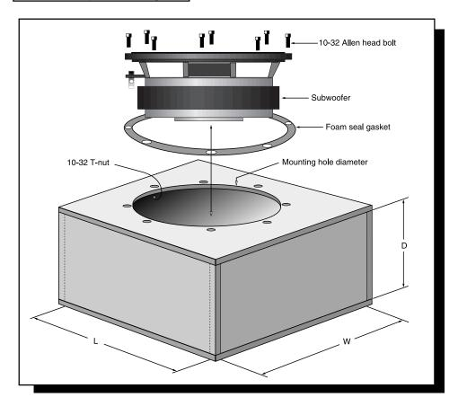
Internal dimensions should be calculated to determine the correct box volume. Be sure to allow for speaker displacement and extra bracing (if used).
