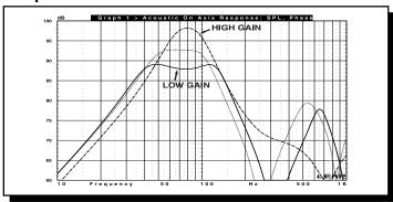
\*ACTUAL IN-CAR RESPONSE CURVE WILL VARY BASED ON CAR TYPE, WOOFER LOADING, AND ENCLOSURE DESIGN.
