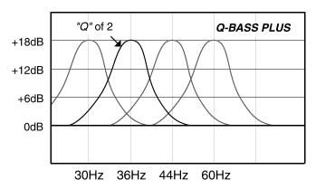
**CAUTION:** *QBASS PLUS*<sup>™</sup> should only be used in systems with a strong subwoofer section. +18dB is a tremendous amount of bass boost and may damage your speakers or create excessive distortion if abused.
