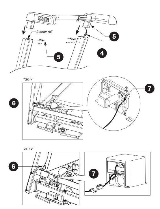
Unwrap the cable and remove the kinks. Ask your assistant to hold the handrail extensions while you feed the cable inside the right upright support. Make sure the cable connector rests on the floor at the base of the upright support.
