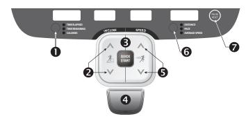
Diagram 12: Lower Display keypad and the Selection keys
