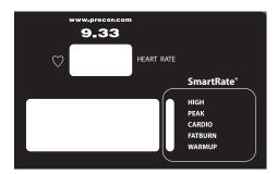
Heart rate and SmartRate® features are available when you wear the chest strap or grasp both touch-sensitive grips (9.33 only). When a heartbeat is detected, the HEART RATE display shows your heart rate and, if your age has been entered, the SmartRate LED pulses and indicates your target zone.
