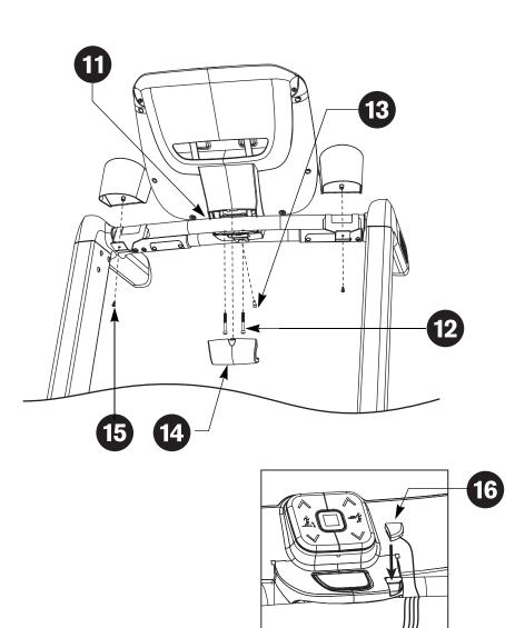
Position the display console so the half-round cutout rests on the display support bar. Place any excess cables inside the display console. Tip the display console up so its base aligns with the mounting bracket on the center handrail.
