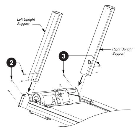
CAUTION: The location of the On/Off switch is beneath the cutout on the base frame. Make sure the power switch is in the Off position. Make sure the power cord is disconnected from its power source.
