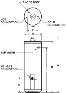
\*Location for optional top-mounted T&P Valve, if ordered from factory. To order, add "G" to model number (GPX 40 YXRTG)
