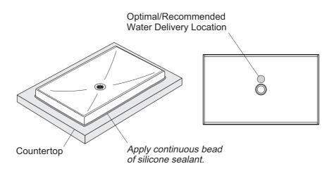
**Important!** When installing the tap, the water should contact the basin in the area shown in the diagram for best performance.
