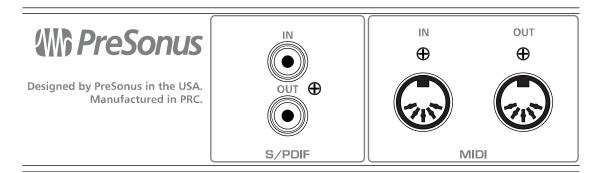
• <u>S/PDIF In and Out Jacks.</u> These allow the FireStudio Project to receive and transmit audio from other digital audio devices. The S/PDIF standard allows two channels of audio to be transmitted at rates up to 24bit/96kHz. The S/PDIF input also allows the FireStudio Project to receive Word Clock – the synchronizing signal indicating the sampling frequency or rate of sample words over a digital interface.
