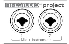
• <u>Instrument Inputs (Channels 1 and 2)</u>. The ¼" TS connector on channels 1 and 2 are for use with an instrument (guitar, bass, etc.). When an instrument is plugged into the instrument input, the microphone preamp is bypassed, and the FireStudio Project becomes an active instrument preamplifier.
